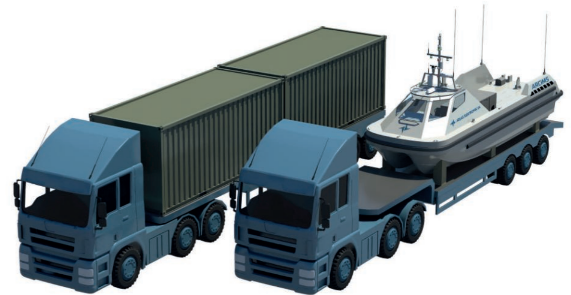
ARCIMS can be simply transported into theatre using a containerised method
