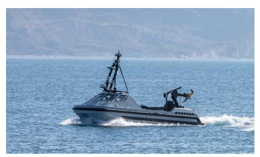
RNMB HARRIER provides sophisticated route survey capabilities and has the ability to launch and recover a range of mission systems including sonars, Autonomous Underwater Vehicles and Remote Operating Vehicles
